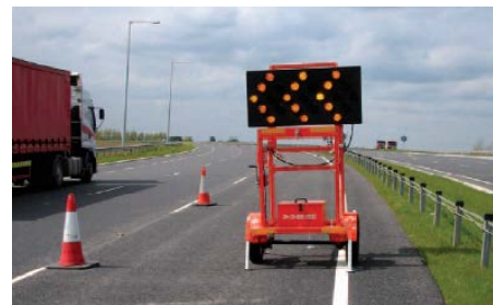
Figure 3.9: Mobile VMS (Displaying Chevrons)
