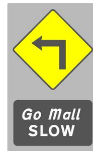
Figure 3.14: Vehicle Activated Sign for Sharp Bend (Sign W 050L with SLOW)
